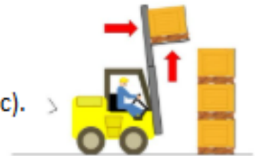
(b) Slow down, stop at the face of stack. Raise the load to the desired stacking!
